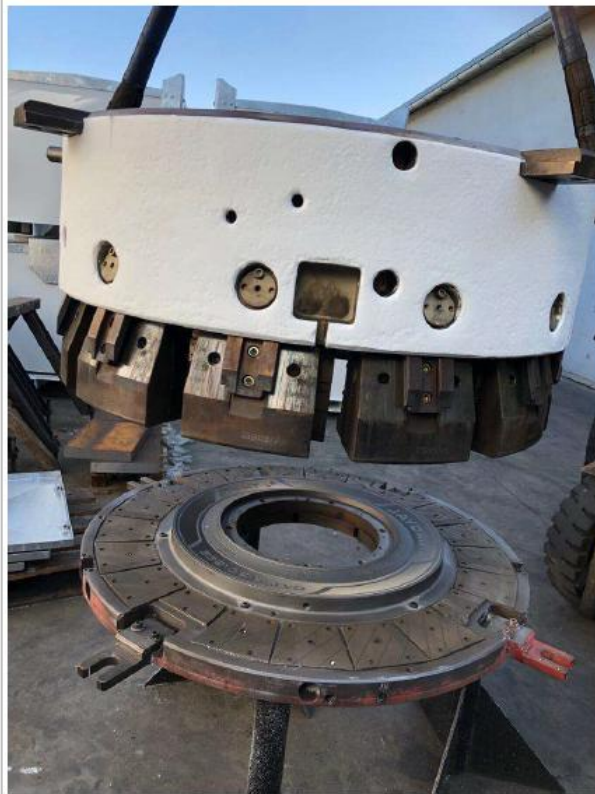
Application of insulation coating - PSCoat:
