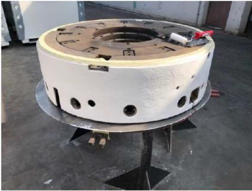
Application of insulation coating - PSCoat:
